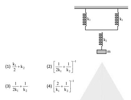
Q.10 Some springs are combined in series and parallel arrangement as shown in the figure and a mass m is suspended from them. The ratio of their frequencies will be:
